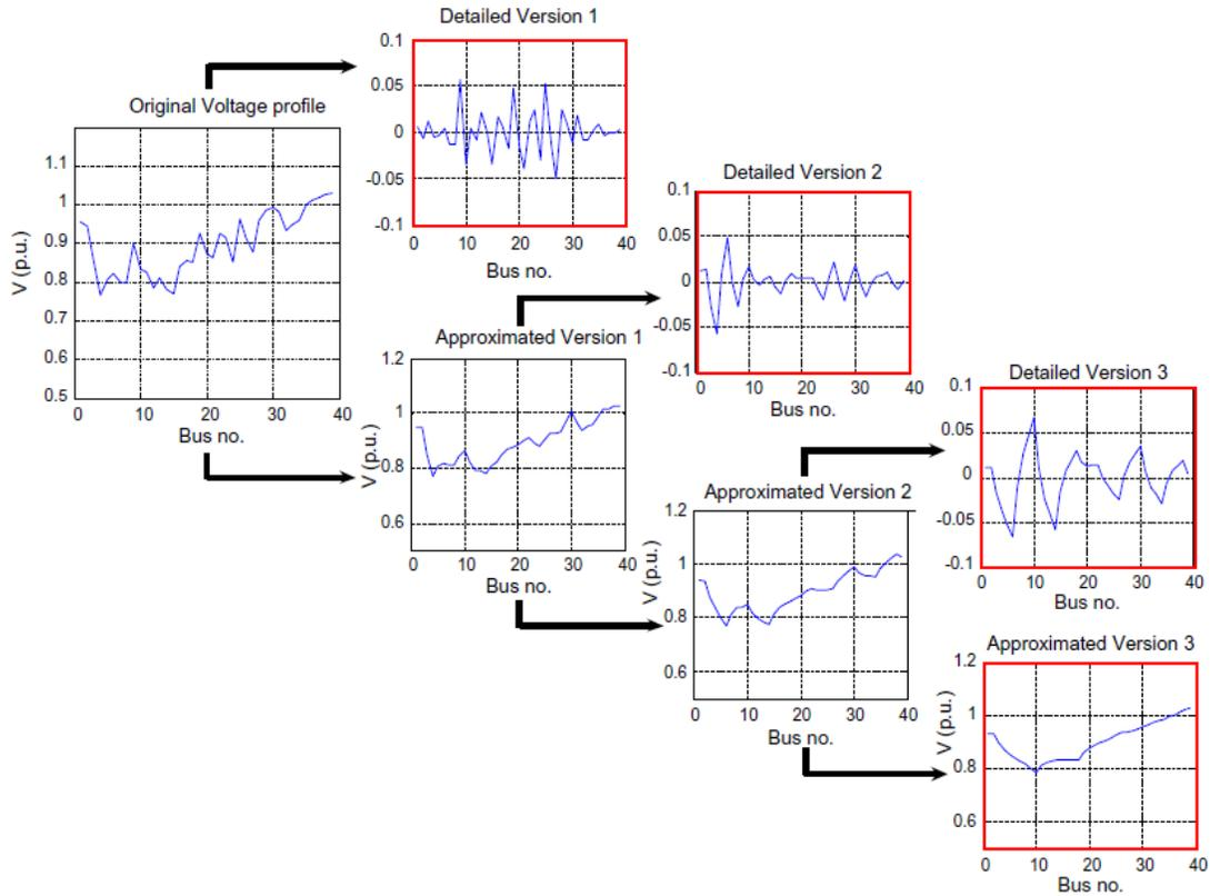
**Figure 4: The feature extraction procedure using wavelet transform**
