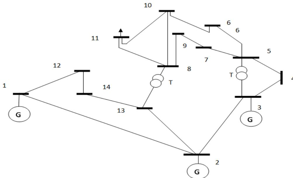
Figure 6: The 14-node test power network
