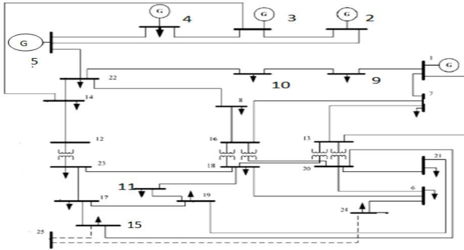
**Figure 7: The 25-node test power network**
