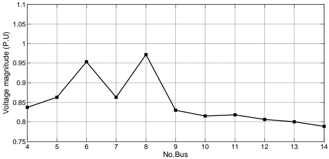
**Figure 8: The voltage profile of test system (14- node)**
