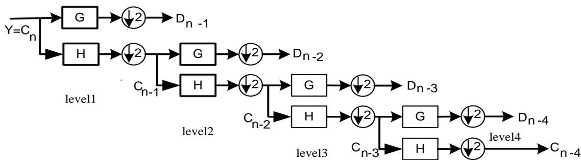
**Figure 1: Multi resolution decomposition of signal Y**
