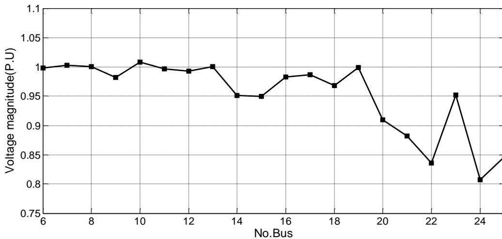
**Figure 9: The voltage profile of test system (25- node)**
