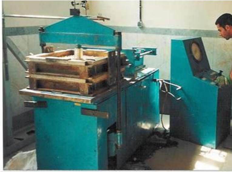
Figure 6: Plate load test apparatus
