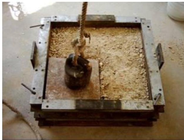
**Figure 5: Tamping and Dynamic compaction of samples**
