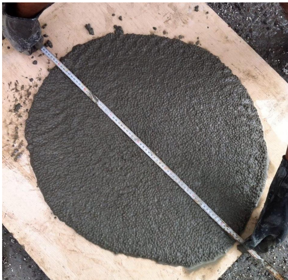
Figure 2: Slump test on the concrete containing coarse EPS
