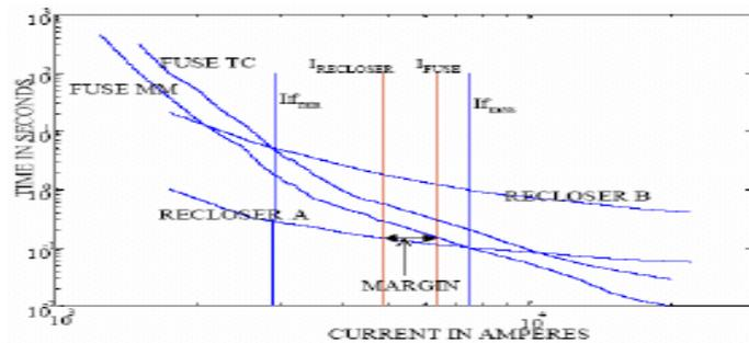
**Figure 5: Coordinating range of fuse reclosing**
