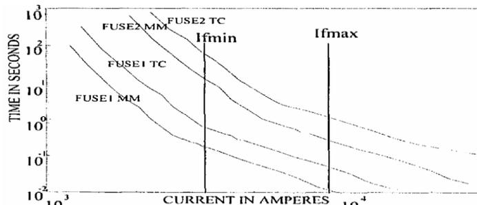
**Figure 1-B: Coordination curve of the two fuses**
