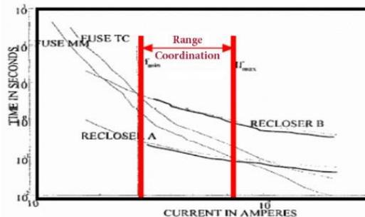
**Figure 4: Coordination range without the presence of DG**
