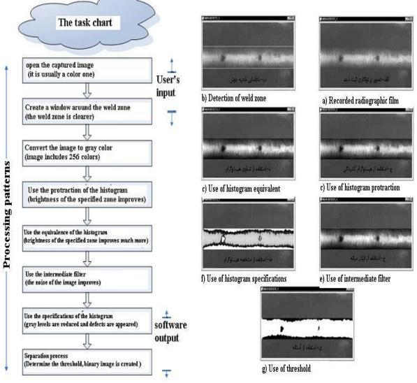
Figure 6: The main algorithms used to detect weld defects; Fig. (7) The results of system performance on images
