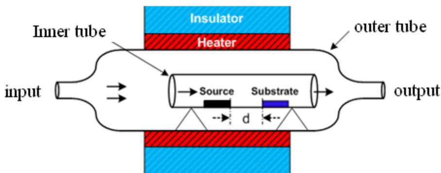
Figure 1: Fabricating nanostructure base on PVD method
