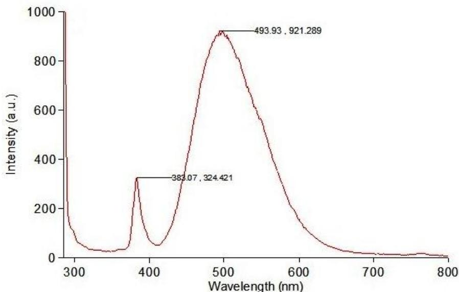
**Figure 5: PL analysis result from fabricated nanostructures without using catalyst**
