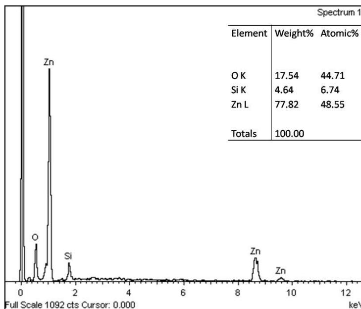
**Figure 4: EDX spectrum which show the equal amount of oxygen and zinc oxide**
