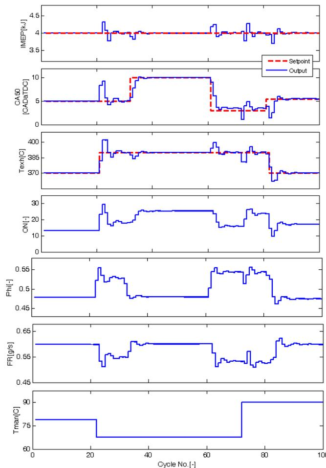
**Figure 9: Disturbance rejection; intake temp. variation of (85-65-100 C)**
