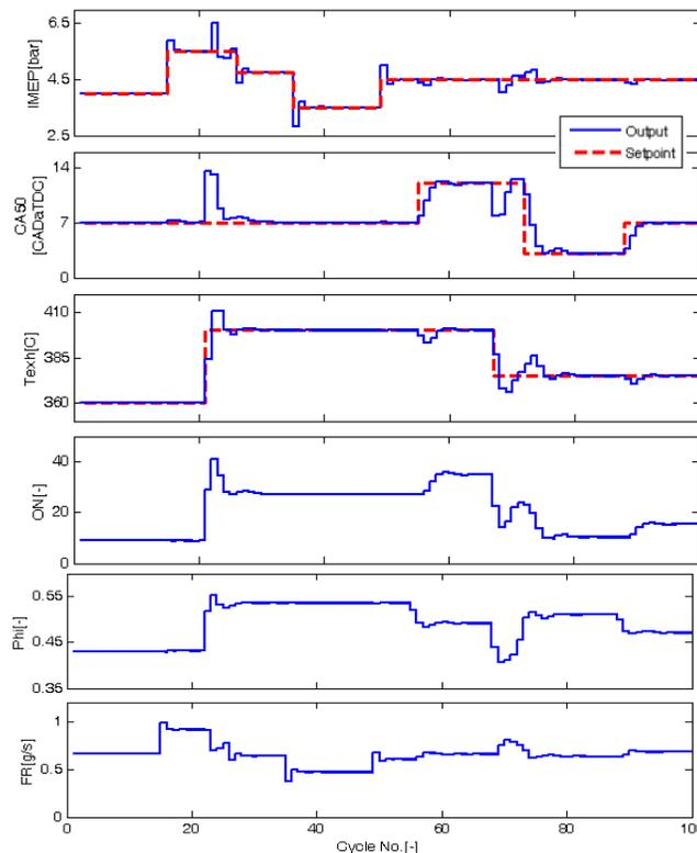
**Figure 7: Single tracking performance for IMEP, CA50 and  $T_{exh}$**
