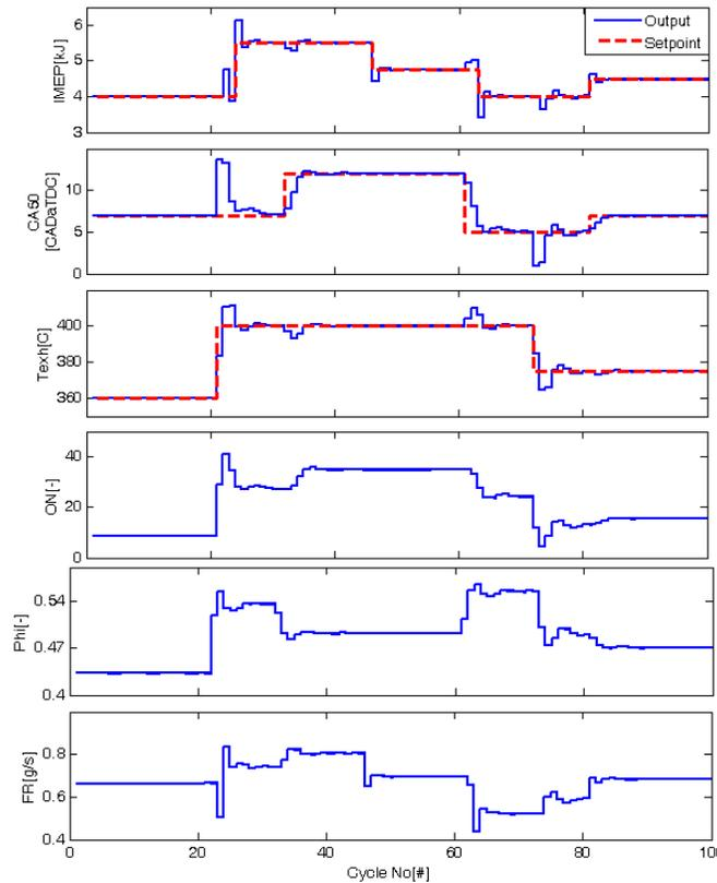
**Figure 8: Simultaneous tracking performance of IMEP, CA50 and**
