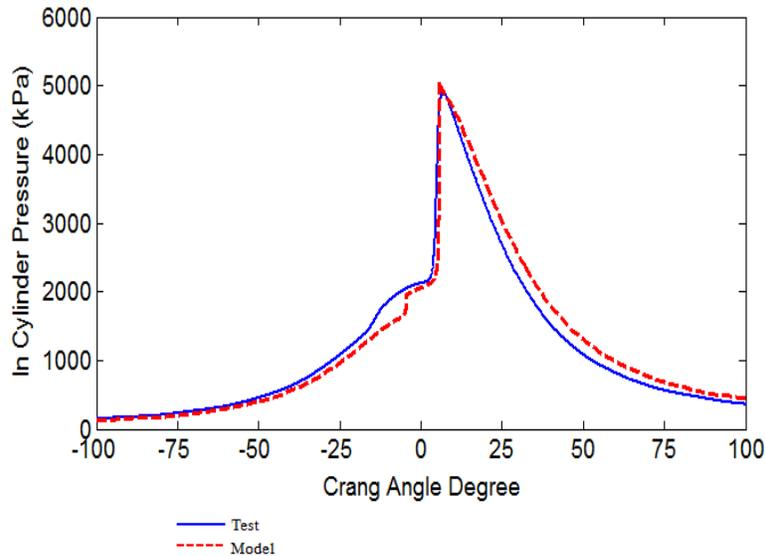
**Figure 1: Comparison of pressure simulated and test No. 3**
