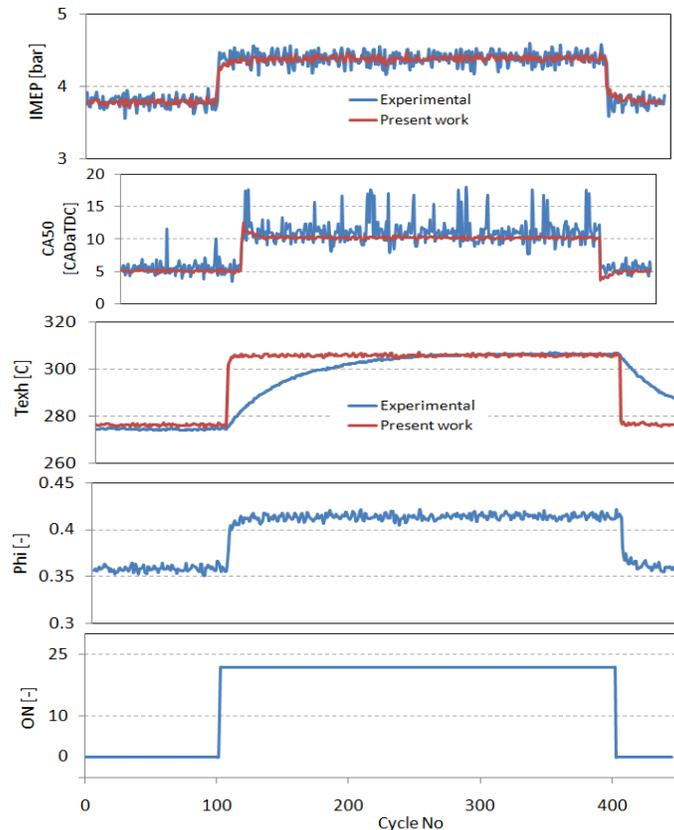
**Figure 4: COM test results validation for a step change in  $\phi$  and ON for 445 engine cycle**
