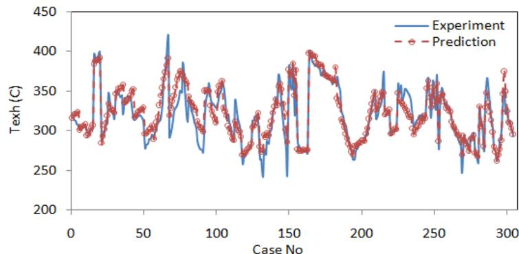
**Figure 3: Comparison between predicted and experimental  $T_{exh}$**
