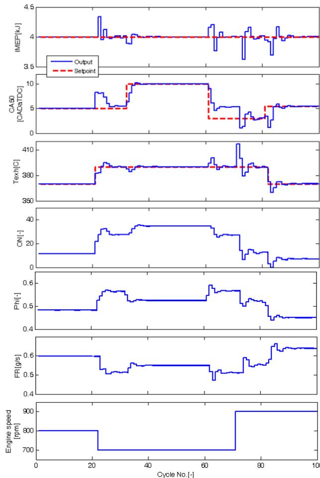
**Figure 10: Disturbance rejection for speed variation (800-700-900 rpm)**
