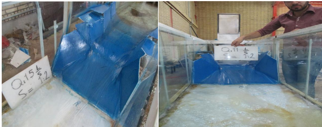
Figure 3: Built Long throat flume with 20 cm sill height and 1:2 slope (experimental)
