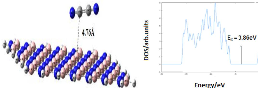
**Figure 2: Cyanogen adsorption on the BNNS and DOS diagram for observing  $E_g$  of nanosheet. Distance is in Å**
