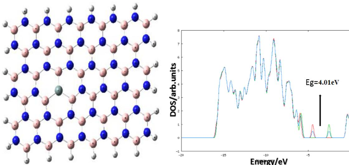
**Figure 5: Doped nanosheet by Si<sub>N</sub> and DOS diagram for E<sub>g</sub> of nanosheet**
