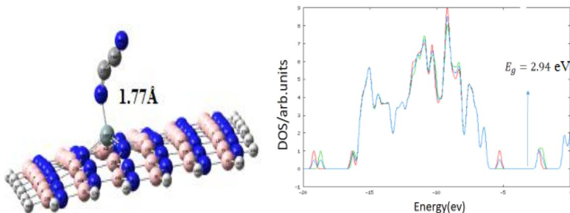
**Figure 6: a) Cyanogen adsorption on doped nanosheet by Si<sub>N</sub> and DOS diagram for observing of E<sub>g</sub> nanosheet. b) Cyanogen adsorption on doped by Si<sub>B</sub> and DOS diagram for observing of E<sub>g</sub> nanosheet. Distance is in Å**
