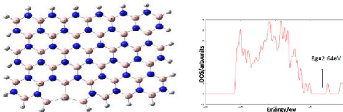
**Figure 3: Doped nanosheet by  $Al_N$  and DOS diagram for  $E_g$  of nanosheet**
