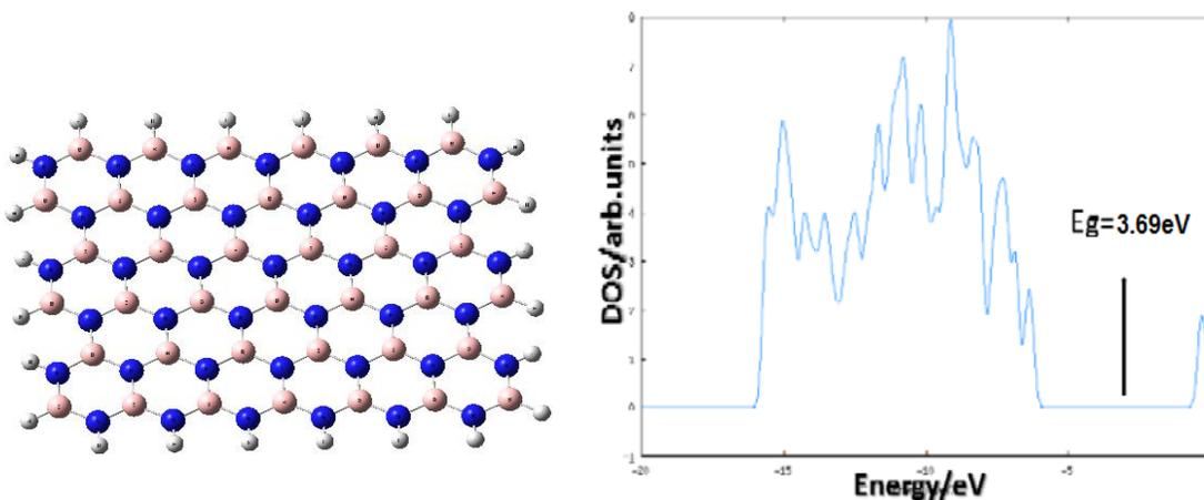
**Figure 1: BNNS and DOS diagram for  $E_g$  of nanosheet**
