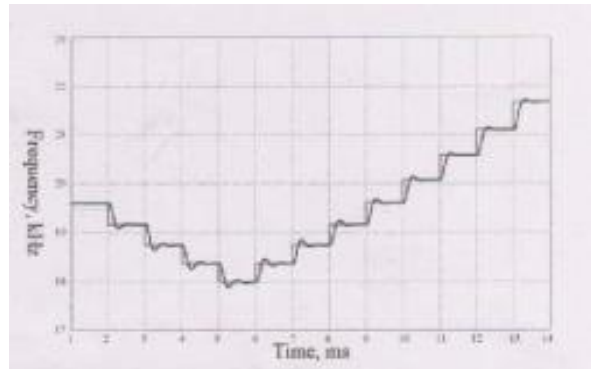
Figure 5: Tracking the changing resonant frequency
