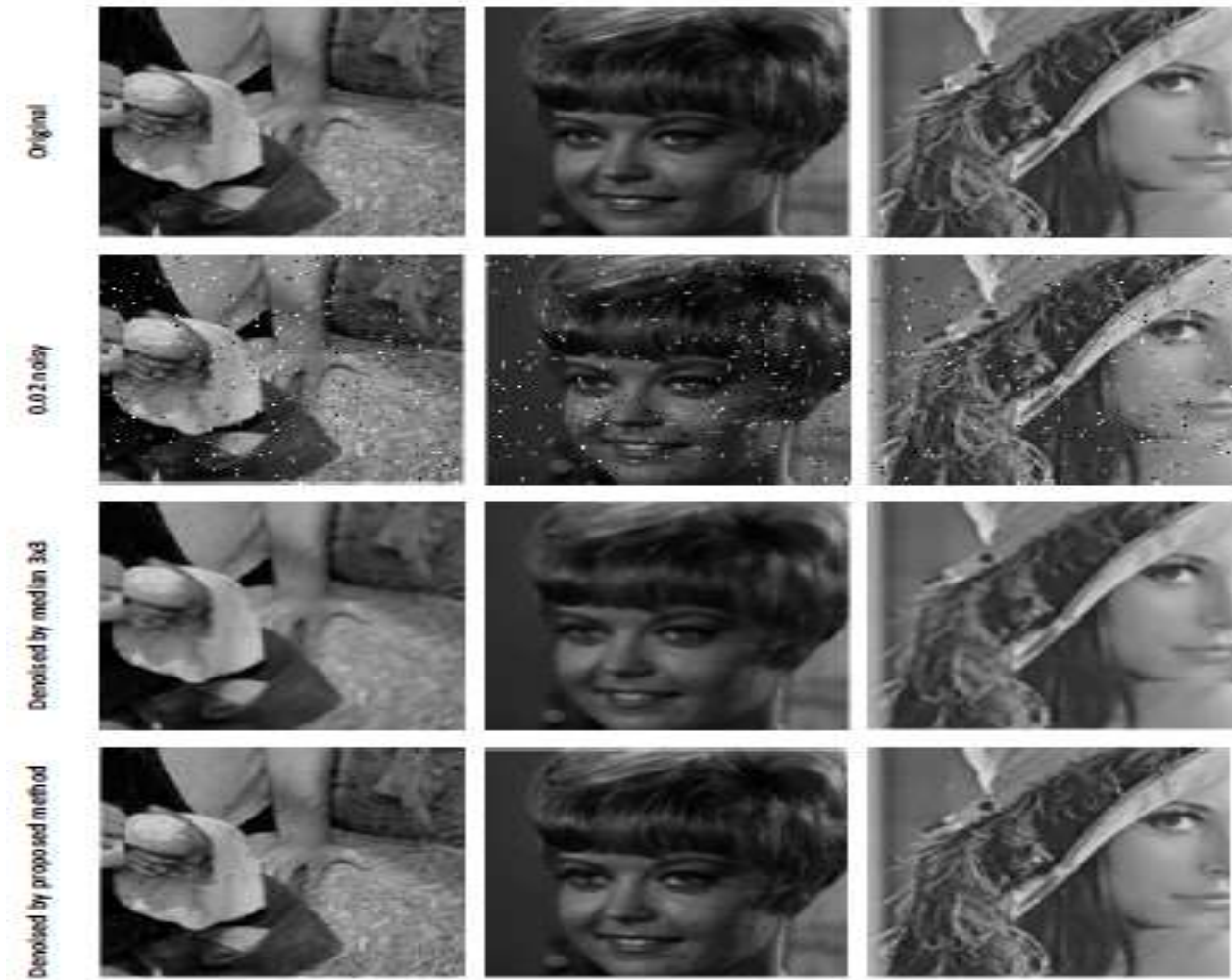
Figure 12: The zoomed view of the cleaned images using denoising by prediction on rows and columns; first row: original image; second row: image corrupted by 0.02 impulse noise; third row: cleaned image using median filter 3x3; fourth row: cleaned image using Neuro-Fuzzy system
