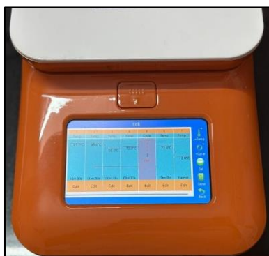
Figure 3. PCR program for the amplification of mtCOI gene.
