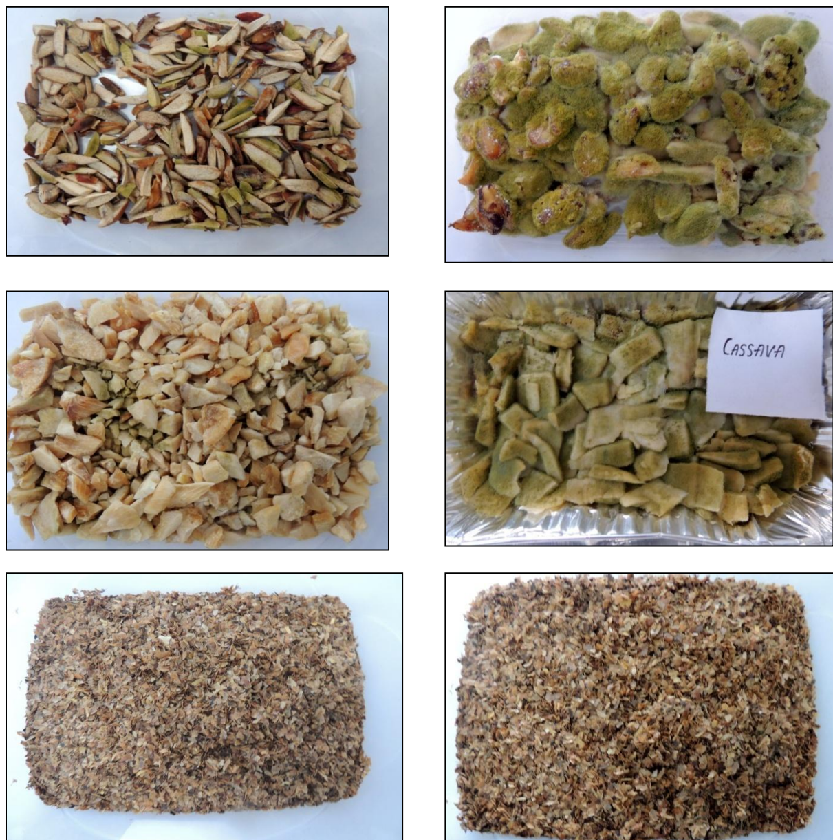
Figure 1: Production of Amylase Using Solid State Fermentation Using Various Substrates, Jackfruit Seeds (Top Left); Boiled Jackfruit Seeds (Top Right); Cassava Peels (Middle Left); Boiled Cassava Peels (Middle Right); Coffee Husks (Bottom Left); Boiled Coffee Husks (Bottom Right)
