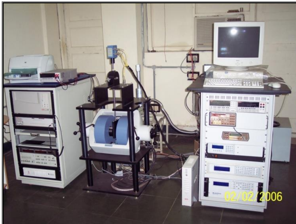
Figure 2: Block diagram of closed cycle refrigerator based cryostat used for I-V-T and low temperature Hall measurement.
