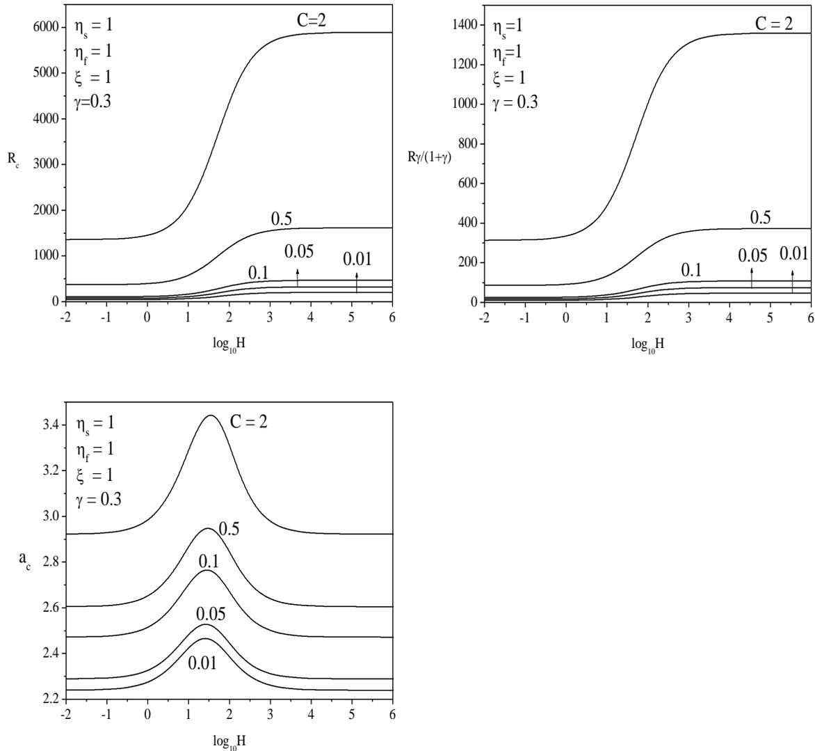
Figure 5. Variation of critical Rayleigh number, critical Rayleigh number based on mean properties of the porous medium and critical wave number with interphase heat transfer coefficient  $H$  for different  $C$
