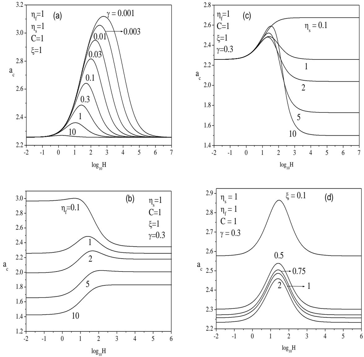
Figure 2. Variation of critical wave number with interphase heat transfer coefficient H for different values of  $\gamma, \zeta, C, \eta_s$  and  $\eta_f$
