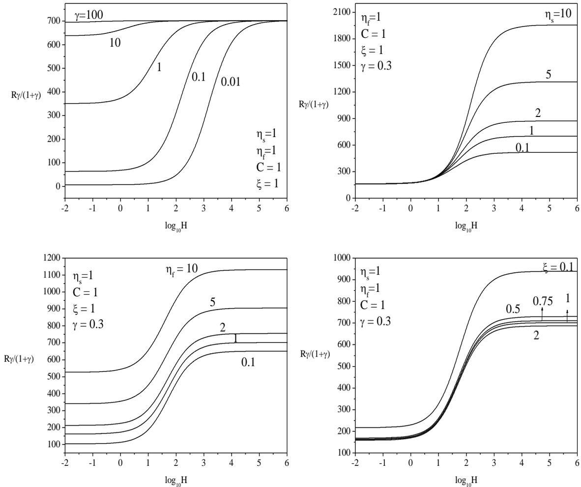
Figure4. Variation of critical Rayleigh number based on mean properties of the porous medium with interphase heat transfer coefficient H for different values of  $\gamma, \zeta, C, \eta_s$  and  $\eta_f$
