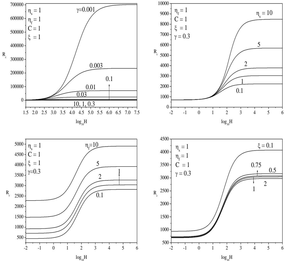
Figure 3. Variation of critical Rayleigh number with interphase heat transfer coefficient  $H$  for different values of  $\gamma$ ,  $\zeta$ ,  $C$ ,  $\eta_s$  and  $\eta_f$
