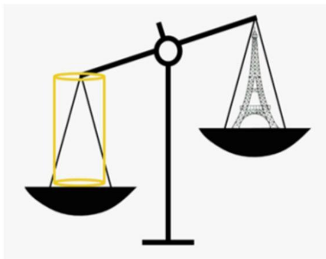
Figure 21: Air Enclosing Eiffel Tower is Heavier than Weight of Eiffel Tower
