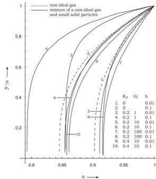
**Figure 6: Variation of reduced density  $\frac{\rho}{\rho_2}$  in the flow-field behind the shock front for  $\bar{\alpha}=0.025$**
