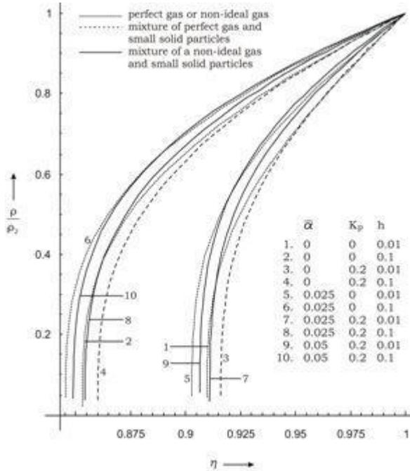
**Figure 3: Variation of reduced density  $\frac{\rho}{\rho_2}$  in the flow-field behind the shock front for  $G_1=10$**
