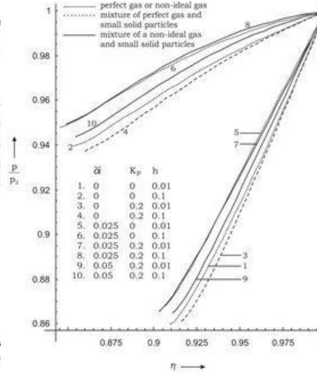
**Figure 2: Variation of reduced pressure  $\frac{p}{p_2}$  in the flow-field behind the shock front for  $G_1 = 10$**
