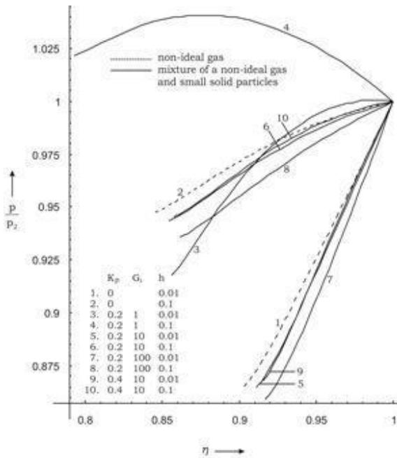
**Figure 5: Variation of reduced pressure  $\frac{p}{p_2}$  in the flow-field behind the shock front for  $\bar{\alpha}=0.025$**
