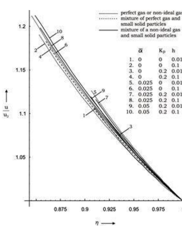
**Figure 1: Variation of reduced velocity  $\frac{u}{u_2}$  in the flow-field behind the shock front for  $G_1 = 10$**
