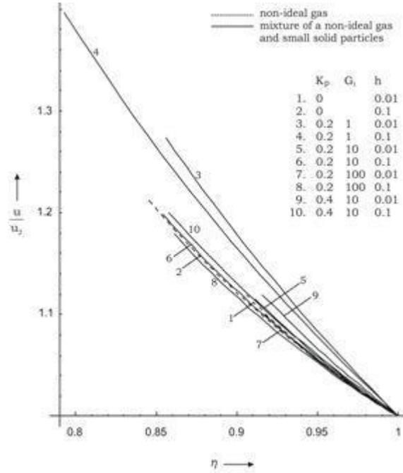
**Figure 4: Variation of reduced velocity  $\frac{u}{u_2}$  in the flow-field behind the shock front for  $\bar{\alpha}=0.025$**
