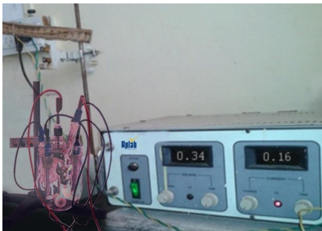
Figure 1.1: Photograph of Schematic of full experimental system with saturated calomel electrode (SCE) Setup
