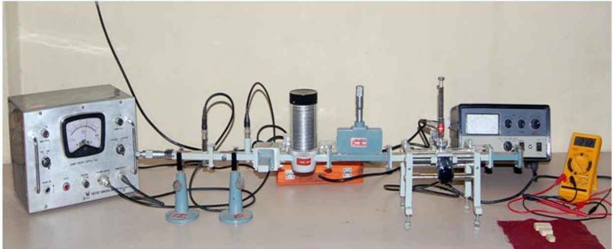
Figure 1: X-band microwave set-up for measuring dielectric constant of wood by waveguide cell method
