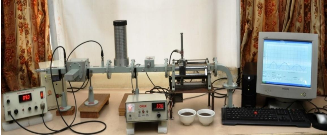
Figure 1: Automated C-Band Microwave Setup for Measurement of Dielectric Constant of Soils
