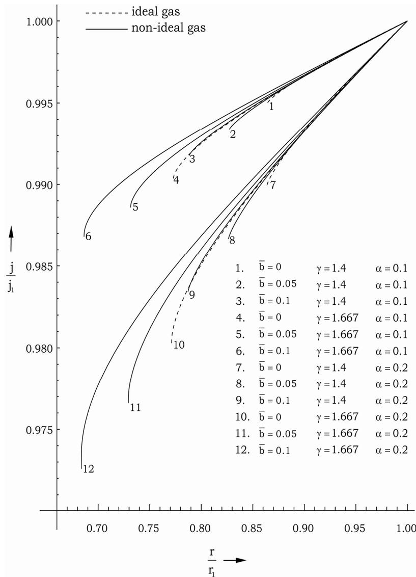
Figure 4: Variation of radiation flux  $j/j_1$  with radial distance  $r/r_1$  in the flow-field behind the shock
