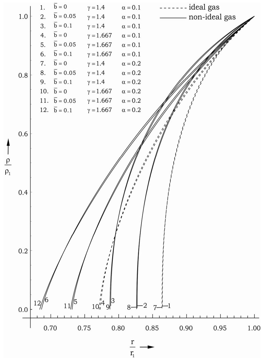
Figure 2: Variation of density  $\rho/\rho_1$  with radial distance  $r/r_1$  in the flow-field behind the shock
