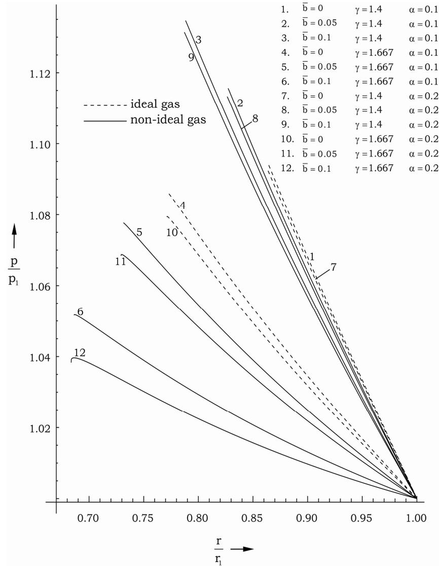
Figure 3: Variation of pressure  $p/p_1$  with radial distance  $r/r_1$  in the flow-field behind the shock
