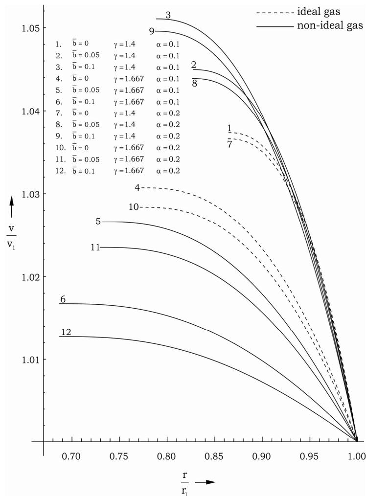
Figure1: Variation of radial fluid velocity  $v/v_1$  with radial distance  $r/r_1$  in the flow-field behind the shock
