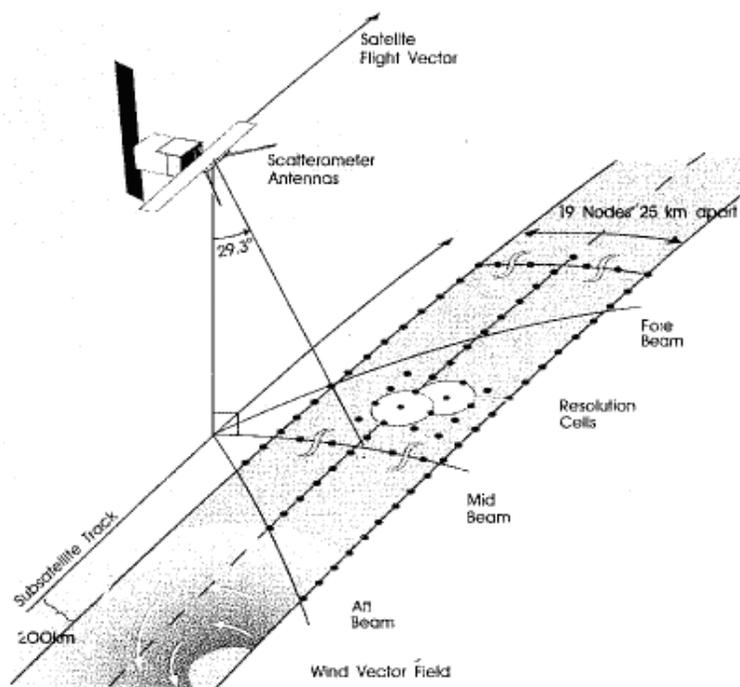
**Figure 2: QuikSCAT wind Scatterometer principle**
