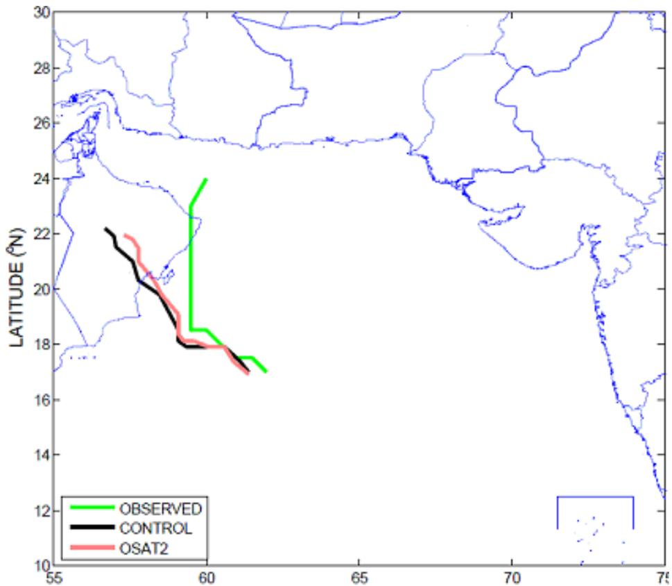
**Figure 13: OCEANSAT – data assimilation in WRF model (OSA2 shows improvement in cyclone track forecast as compared with observed track)**
