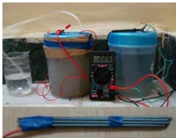
Figure 2: DC-MFC setup and the arrangement of graphite from pencils as electrodes
