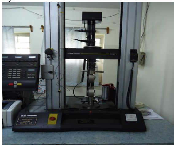
Figure 1: Instron universal testing machine (model 4406)
