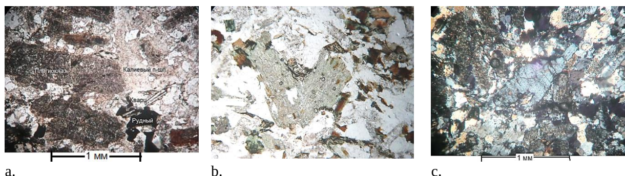
Figure 1. Mineralogical and petrographic characteristics of granodiorites of the main phase in the Southbay mine: a – without analyzer; b, c - with analyzer.
