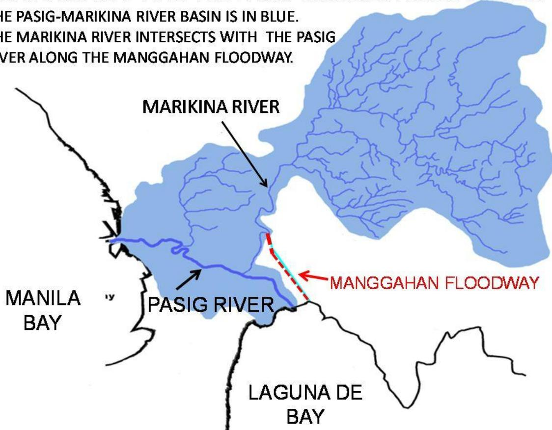
**Figure 3: Drainage map of the Pasig-Marikina River Basin with the Manggahan Floodway shown in red. The Marikina River intersects with the Pasig River along the Manggahan Floodway.**
