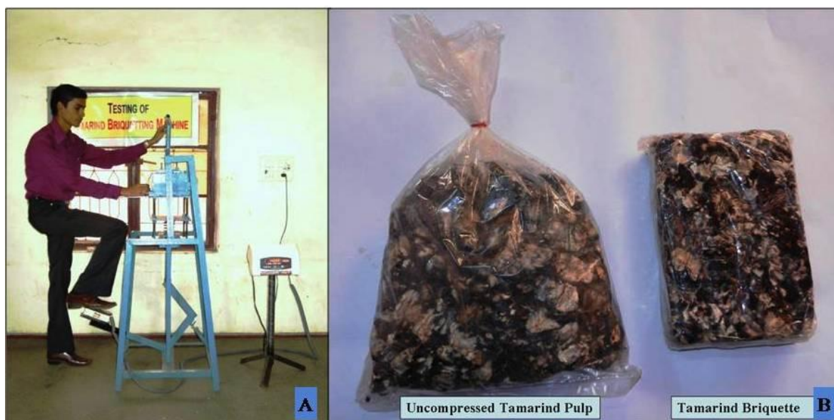
Figure 3: A- Briquetting of tamarind in tamarind briquetting machine, B -Tamarind Briquette
