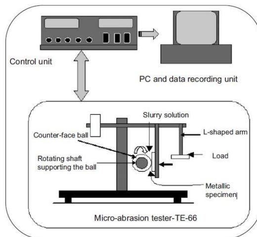
Figure 1. Schematic diagram of microabrasion tester
