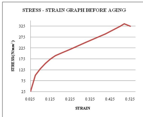
Figure 4(a) Compressive stress of specimen before aging
