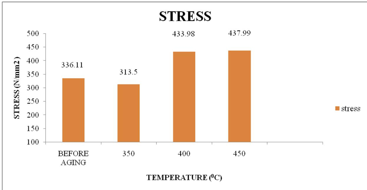
Figure 7 The tensile stress values of specimens before and after aging
