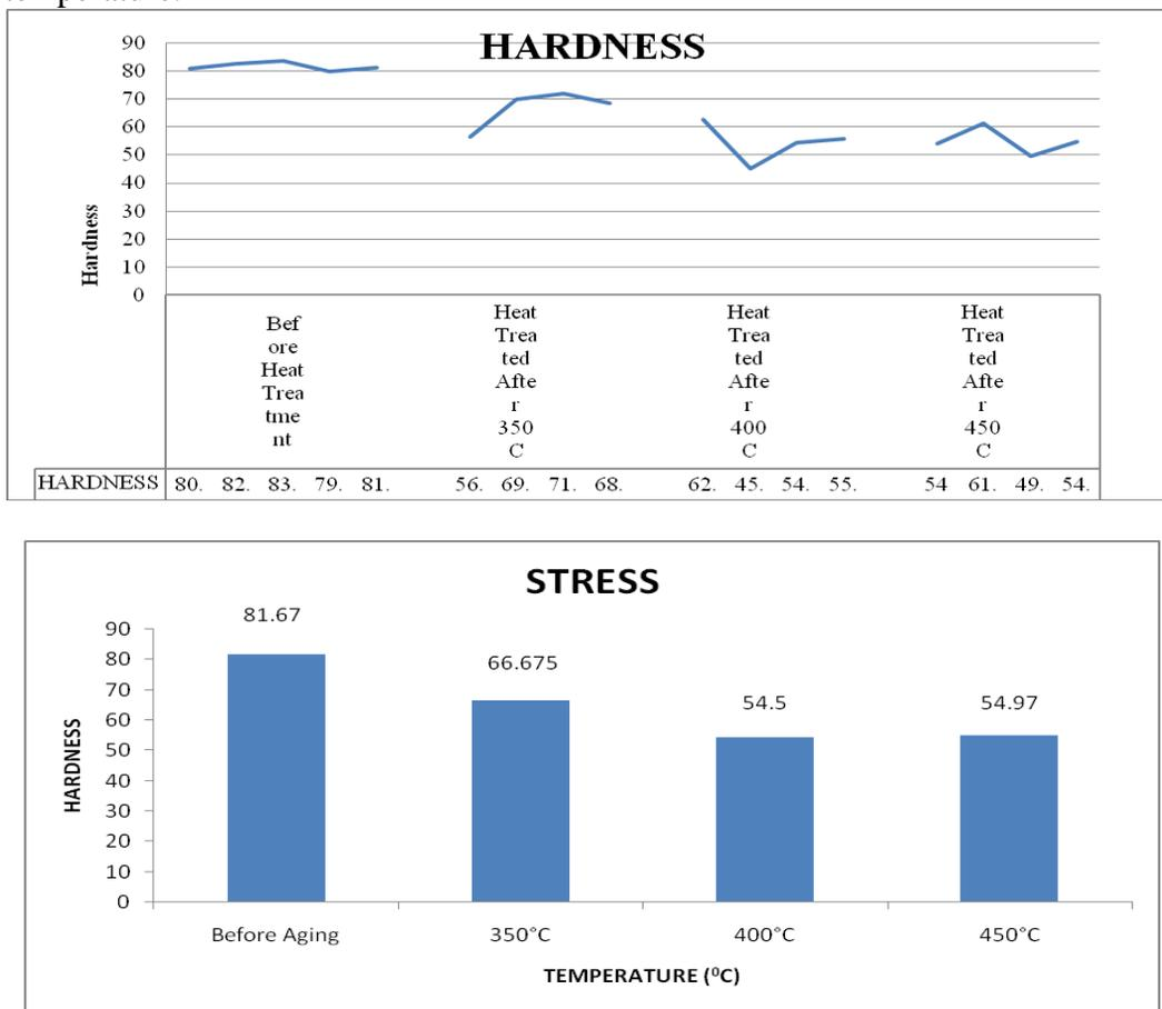
Figure 3: The evaluation of micro hardness values of specimens before and after aging.
