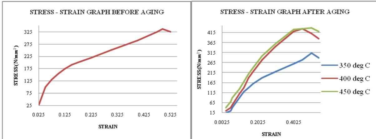
Figure 6(a) Tensile strength of specimen before aging
