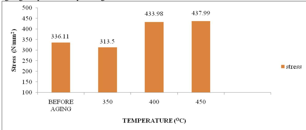
Figure 5. The compressive stress values of specimens before and after aging.
