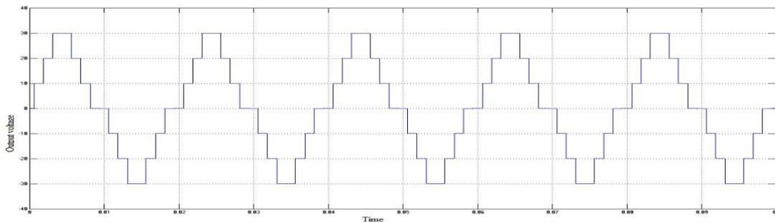
**Figure 5: Seven level output of Multilevel Inverter**
