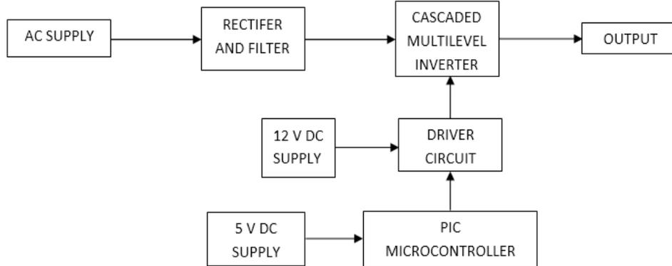
**Figure 2:** Block diagram of Microcontroller based control of CMLI
