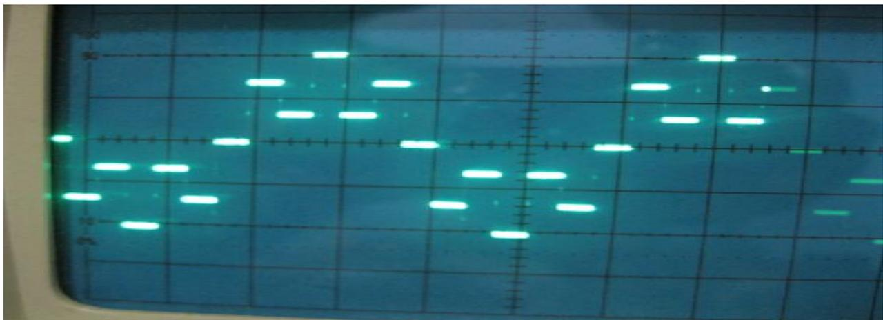
**Figure 8: Seven level hardware output of Multilevel Inverter**
