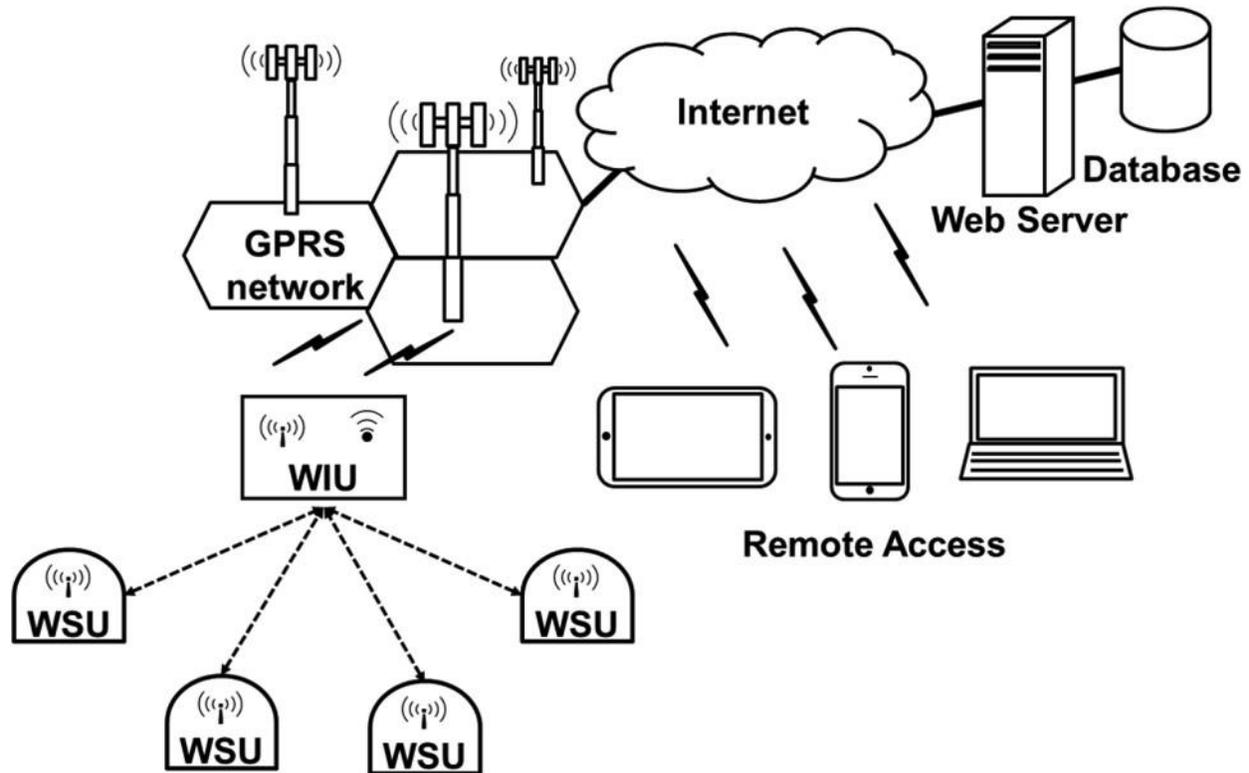
**Fig. 2. Automated irrigation system (configuration of a wireless information unit and wireless sensor units) using WSN, ZigBee, and GPRS (Gutiérrez et al.,2014).**
