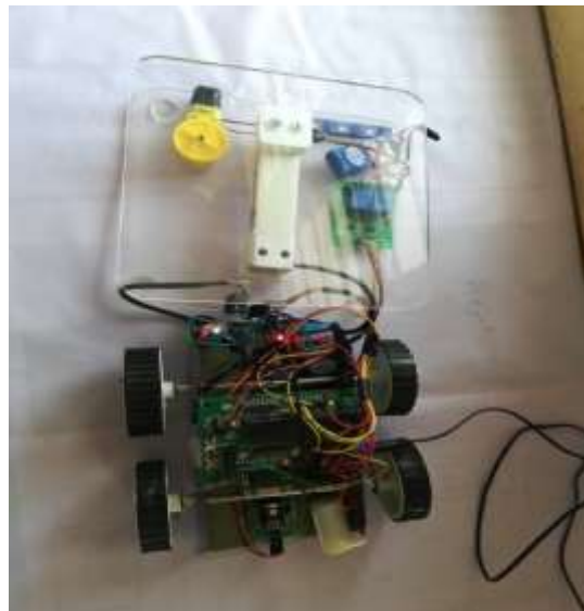
Fig 8: If load is not present, Lights & fans are automatically switched off.
