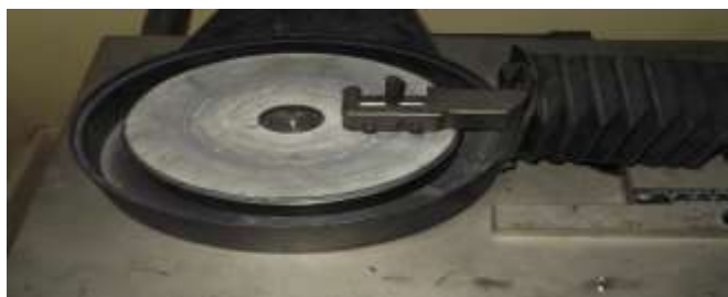
Fig .3 Pin on disc arrangement used for the surface wear study
