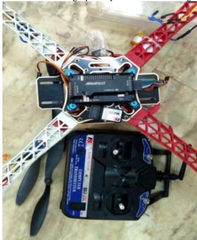
Figure 3b: The APM 2.8 Flight Control Board
