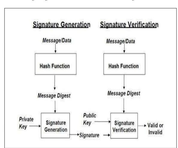
**Digital Signature Generation and Verification Flow Diagram:**
