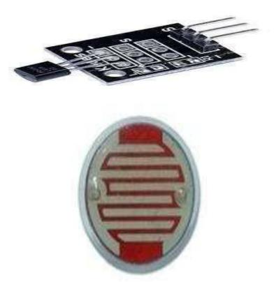
LDR sensor: Light Dependent Resistor or photocell is a light-controlled variable resistor. When the intensity of light increases the resistance of the sensor decreases and vice versa. The LDR should be exposed to light hence it must be placed in a way that the opposite car's light approaching you must fall on the LDR and not on your own car's light.
