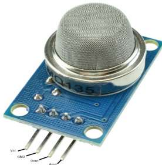
Figure 3: MQ135 Air quality sensor
