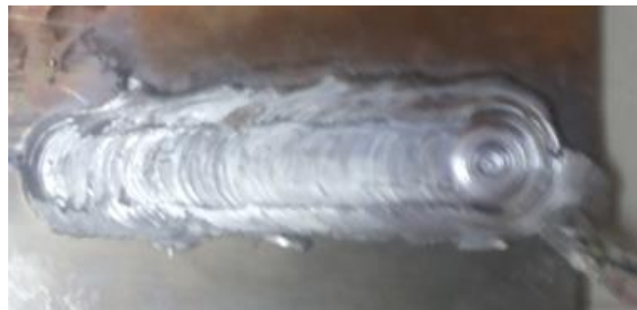
Figure 3: Picture of Plunge Depth as Defect in FSW
