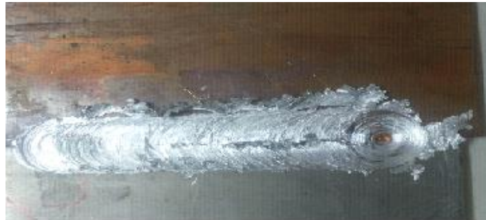
Figure 2: Photo of a Weld Flash with an Additional Surface
