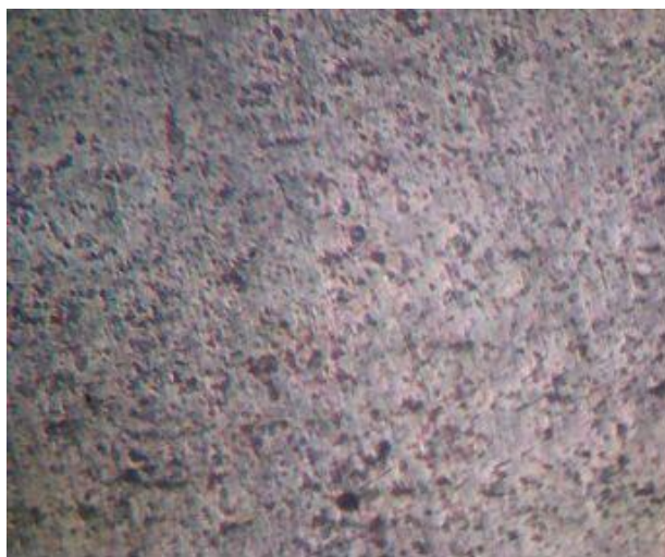
Figure 5: Micrograph of MMC (Al 356 Alloy with 20 % Reinforcement)
