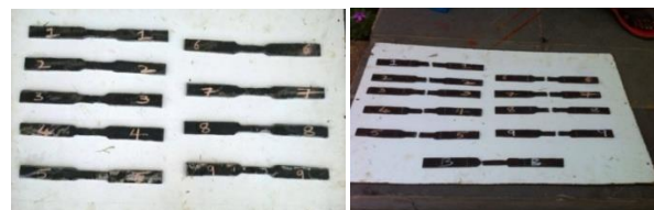
Figure 2: Specimens before & after Tensile Strength Test
