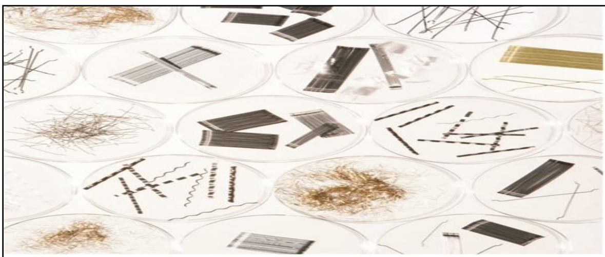
Figure 5: Different types of steel fibres (Source: IRC (2013), Kumar et al., (2014) )
