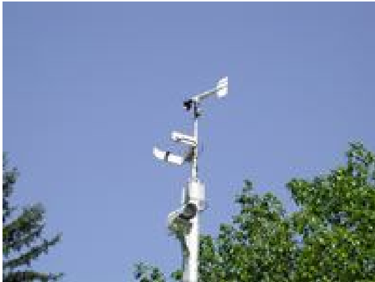
Figure 2: Wind speed/direction sensor (top), precipitation gauge (middle), and fixed-zoom camera (bottom) (Source: ALASKA'S road weather information system. www.alaska.gov )
