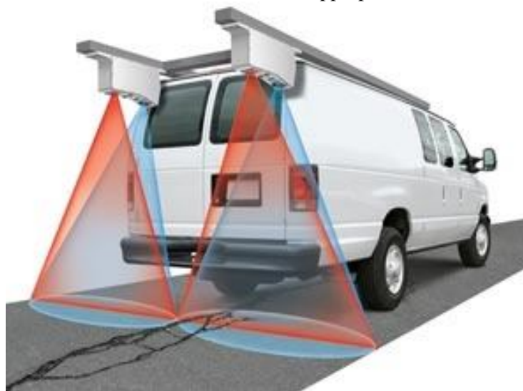
Figure1: Weathering and Raveling Measurement Tool Taken from Aasho Road Test
