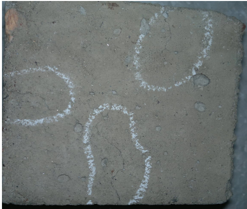
Figure 4: Cracks in B series at 750
