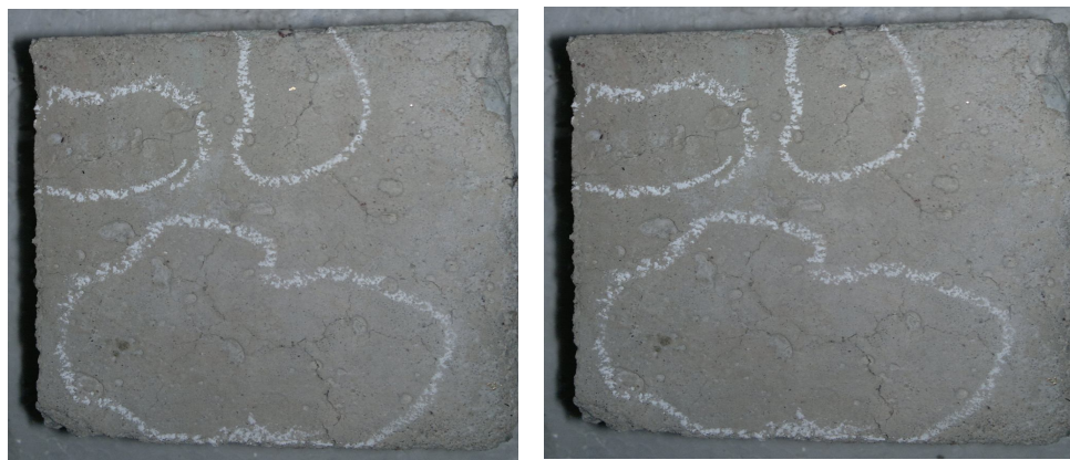
Figure 3: Cracks in OPC (series A) at 750°C
