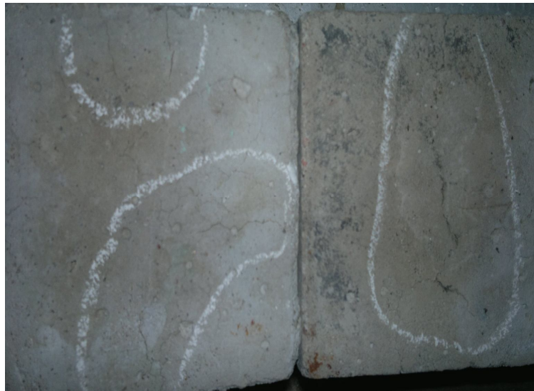
Figure 6: Cracks in Series D at 750°C
