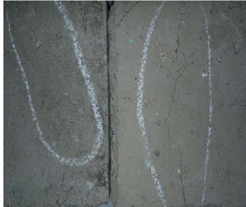
Figure 5: Cracks in Series C at 750°C
