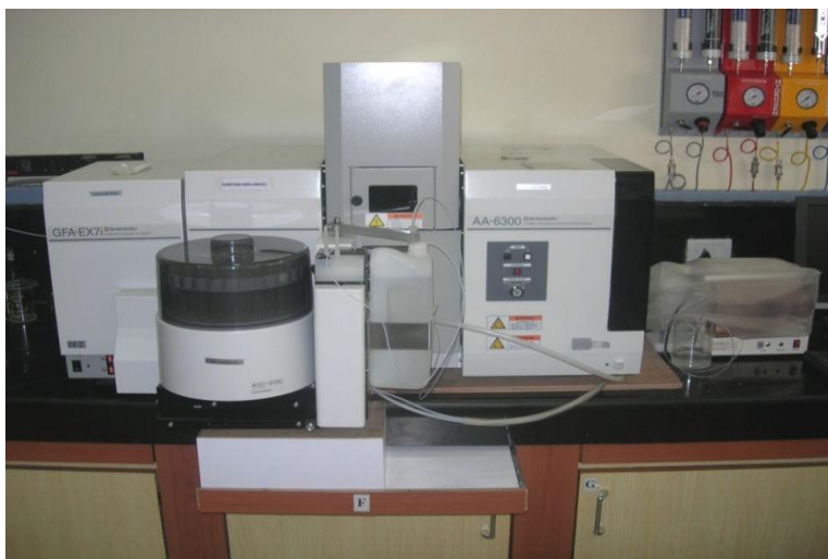
Plate 3: Atomic Absorption Spectrophotometer (AAS) Make- Shimadzu, Model –AA6300
