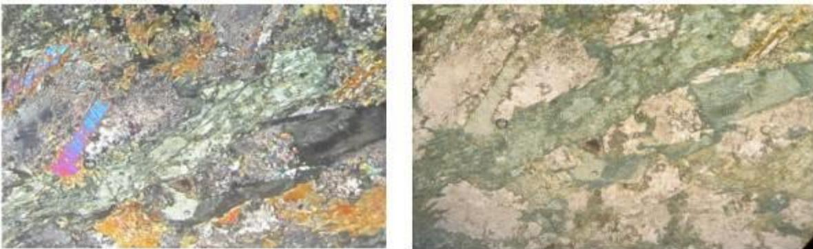
**Figure 10: Hornblende, Apatite, Opaque, Hornblende in Diorite Epidote Stone**
