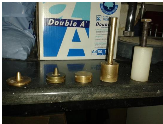
The pin-hole device components
