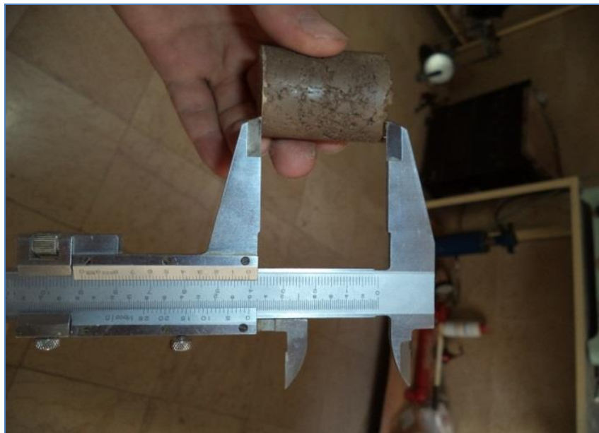
Figure 2-4: Standard length of sample for pinhole test
