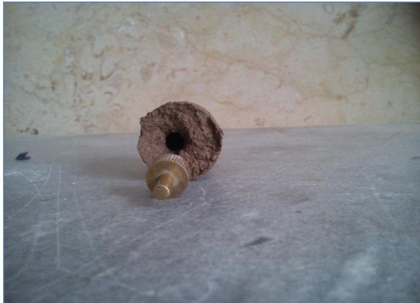
Figure 1-4: Diameter of soil sample after conducting pinhole test
