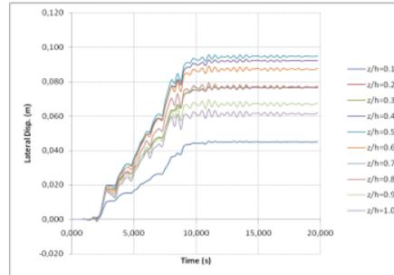
**Figure...: Embankment Horizontal Displacement Time History at Different Levels (Simulation H1)**
