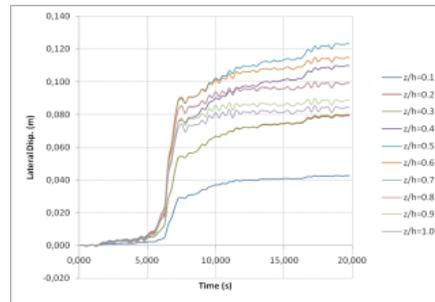
**Figure...: Embankment Horizontal Displacement Time History at Different Levels (Simulation H3)**
