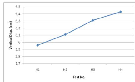
**Figure ...: Vertical Displacement in the Center of Soil Slope (Simulation H1 to H4)**
