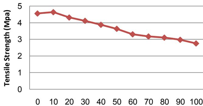
**Figure 7: Tensile strength changes of concrete samples versus freeze-thaw cycles**
