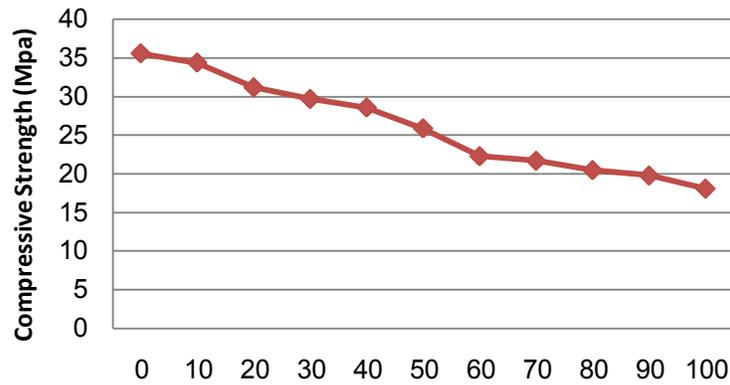
**Figure 6: Compressive strength changes of concrete samples in association to freezing and thaw cycles**
