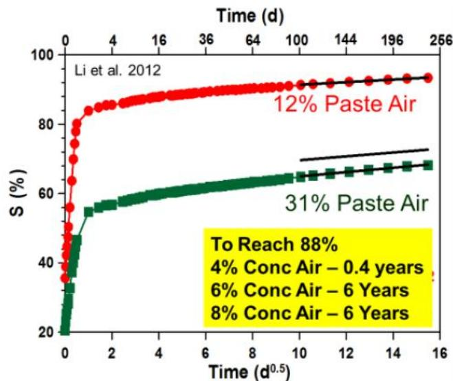
**Figure 2: The required time for reaching critical saturation degree for concrete with different air percentage (Li et al., 2012)**
