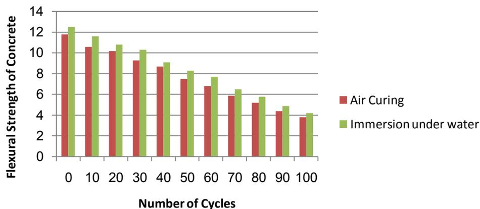
**Figure 9: Comparing the impact of samples curing processes on flexural strength of concrete in different freeze-thaw cycles**
