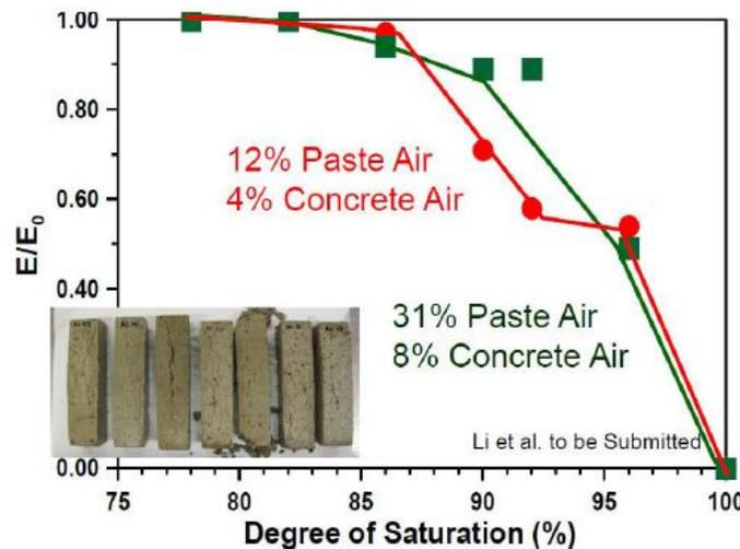
**Figure 1: The relationship between degree of saturation and freeze-thaw duration (Li et al., 2012)**
