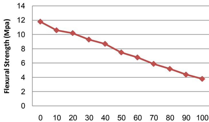
**Figure 8: Flexural strength changes of concrete samples versus freeze-thaw cycles**
