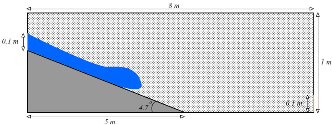
**Figure 6: Schematic of density current**
