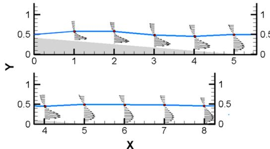
**Figure 13: The diagram of current height and velocity vectors at different sections of the reservoir**
