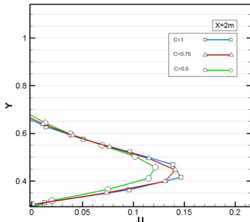
**Figure 9: Velocity profile in different input concentrations**
