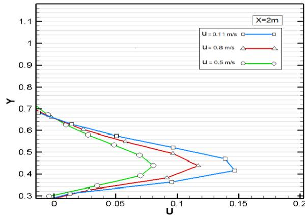
**Figure 12: Velocity profile in different input velocity**
