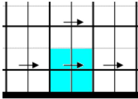
**Figure 5: The horizontal velocity calculation cell adjacent to southern boundary, current bed**
