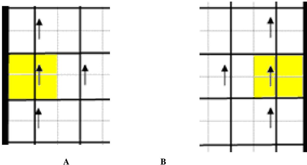
**Figure 4: Vertical velocity cells adjacent to eastern boundary (Figure A) and western boundary (Figure B) or the calculation area**
